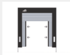
Option: additional removable reinforcement with Velcro system.
