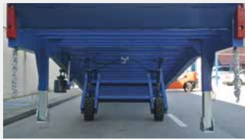
Support and safety feet (rest position). Larger wheels to ensure greater stability.
