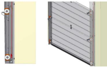
Guide the cable at the lower panel, behind the rollers, to the drums above the door opening. Secure the cable by pushing the cable through the hole in the drum and tightening the hex head screw. Turn the drum until the cable is tight.
